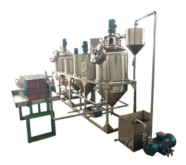
Degumming refers to the degumming treatment of crude edible oil. The specific process is to heat the crude edible oil to 50-70°C and then add phosphoric acid solution to degumming reaction, stir for 30-60min, stir at 50-80rpm, and centrifuge to obtain degummed wool. oil.
