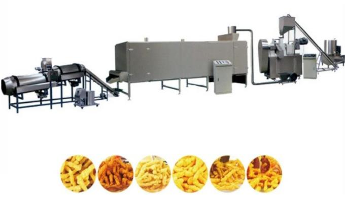
As shown in the picture, it is the **Kurkure Production Line**. This line is from raw material mixing to finished product packaging assembly line production. A whole production line completes all processes. It has a high degree of automation and is very simple to operate. It can greatly save manpower and improve work efficiency. Processing brings great convenience, and its main features are as follows.
