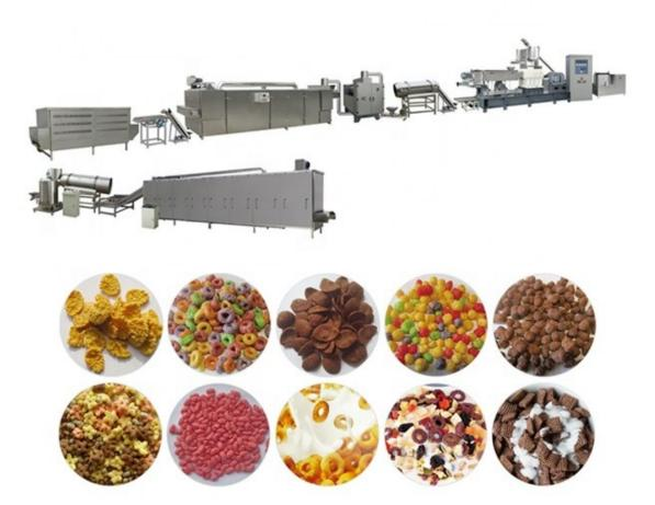
The reason why expanded corn flakes have so many benefits is that they are produced using an advanced twin-screw extruder. The application of extrusion technology is of great significance in the food processing industry.
