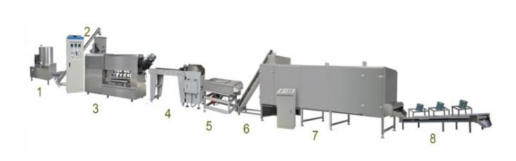
Industrial Macaroni Pasta Production Line consists of a mixing system, an extrusion system, a cutting system, a drying system, a cooling system and a packaging system. Its components include a mixer, a screw conveyor, a screw extruder, a dryer, a cooler, and a packaging machine. The main features of the equipment are as follows:
