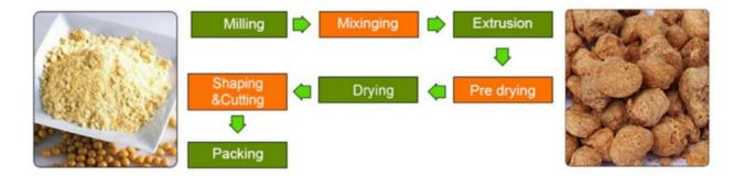
The edible soybean meal is processed into defatted soybean powder through a worm wheel grinder, and the defatted soybean powder that meets the specifications is mixed with 25-30% process water to enter the extruder. In this process, the soybean product is squeezed in a spiral shape under high temperature and high pressure from 20% of moisture, and then rapidly squeezed out of atmospheric pressure to become a dry soybean product by soya bari machine.
