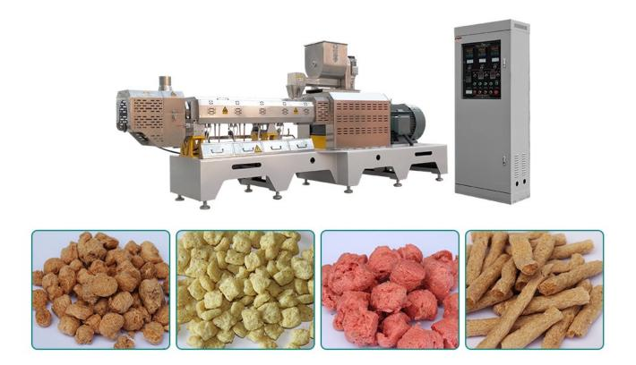
Full fat soya extruder machine can produce different protein content products by changing formulations. Soya bari manufacturing plant produce a kind of vegetarianism with meat like flavor and texture taste, also known as tissue protein. You can get different structure and different shapes protein products, such as soya nuggets, soya chunks, soya mince, etc.
