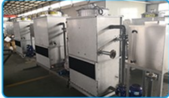
Closed cooling tower
