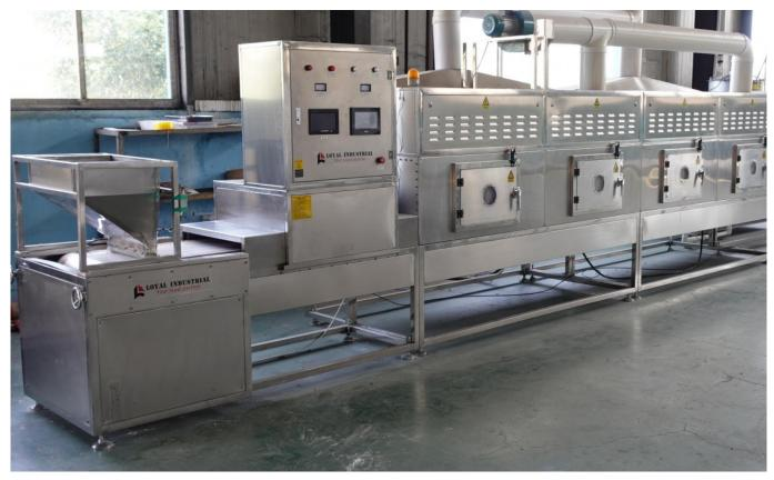
Tunnel Food Microwave Cocoa Powder Beans Powder Sterilization Machine in workshop
