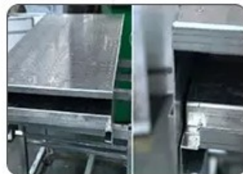
5. Microwave limiter: Prevent microwave leakage
