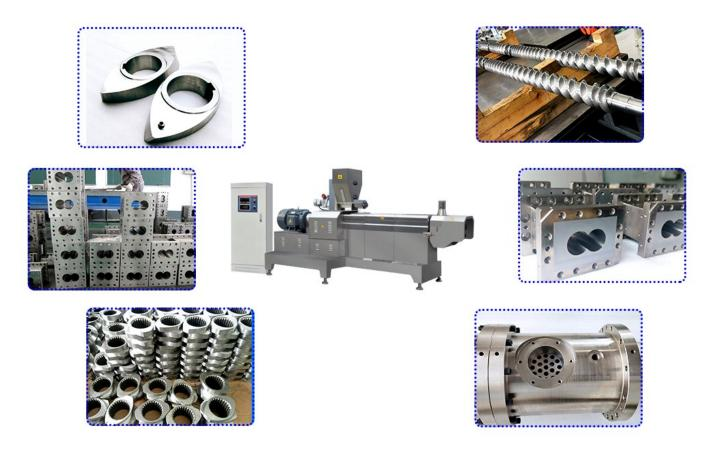
1. The main engine of the industrial pet feed extrusion adopts advanced frequency converter speed regulation technology. It makes the equipment powerful, running more stable and saving electricity. The screw of the feed extruder adopts alloy steel nitriding treatment. And the screw has a longer life. Individual equipment adopts a modular structure. It can be combined according to different needs.
