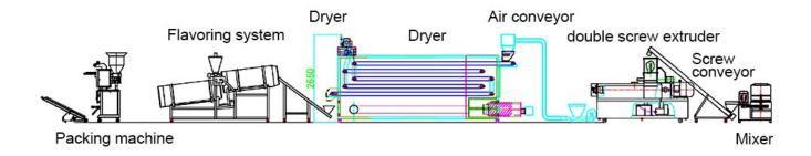
The cavity of the double screw extruder machine adopts a multi-section building block type. Each cavity can independently control the temperature. And there are heating and cooling channels inside. According to user requirements, steam and electric heating methods can be used. The temperature is automatically controlled to control the temperature of the extruder machine product. Convenient, more accurate, to ensure the taste and quality of the twin screw extruder product.
