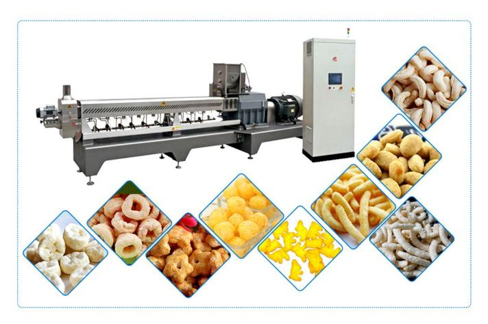
Currently, we sell two types of screw extruder machine. One is a single-screw extruder. And the other is a twin-screw extruder machine. Compared with the former, the advantage of twin screw extruder is relatively more obvious for raw material extrusion and expansion.
