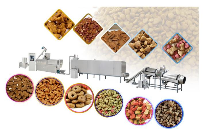
The material can be matured in 10 seconds under the action of the high temperature of the twin screw extruder. And the cooking can be completed in a very short time. It can retain the protein, energy and vitamin content in the material. And it improves the digestibility and palatability of the product.
