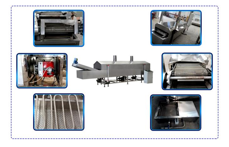
Another more important point is that the fryer must be cleaned after use. The specific method is to wait for the oil to cool and release the oil, then pour in water to boil the water to the boil, and sprinkle in two handfuls of edible alkali powder. Boil for 5-10 minutes, then drain the water.
