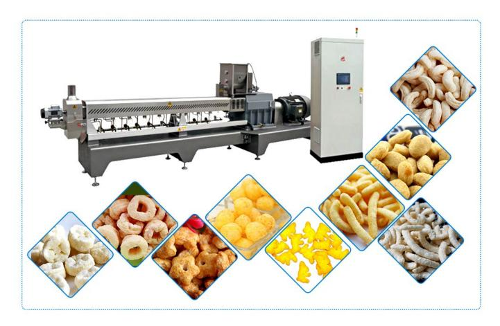
6. According to different product requirements, full automatic double screw extrusion systems with different structures and length-diameter ratios are designed to meet process requirements.
