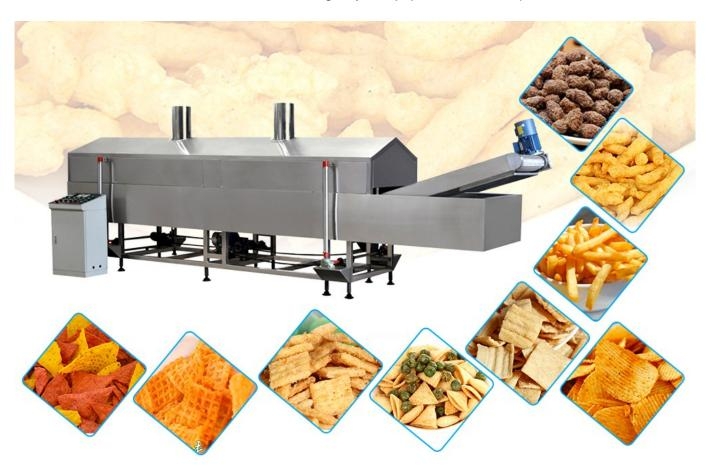
1. The automatic fryer machine adopts advanced technology. It automatically filters impurities in the fryer. This ensures that the frying oil is clean, does not require frequent oil changes. And it reduces the expenditure of raw materials in the frying process. The advanced heating system avoids energy waste to the greatest extent and saves resources.
