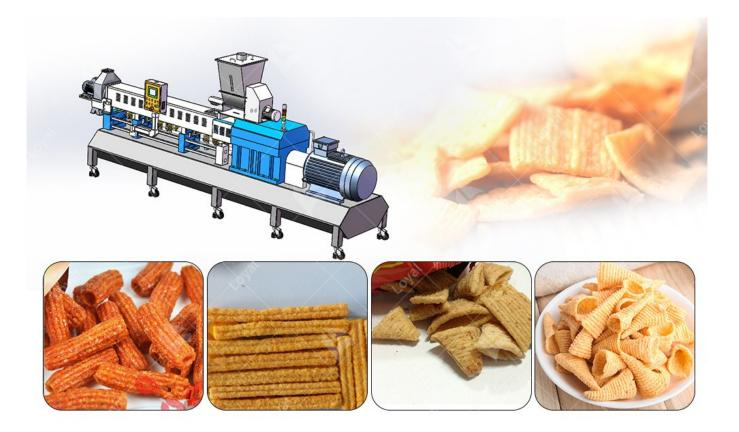
The raw materials can be rice powder, corn powder, wheat flour individually or their mixture. Only by changing the moulds, shaping or cutting machine, the shapes can be various: Sticks, square sheet rib chips, diamond chips, wavy chips, pillow shapes and bugles etc. The taste is good and no greasiness.
