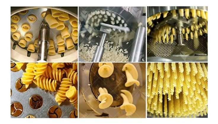
This is indispensable macaroni production equipment for everyone taking on the food profession. Multi-function stainless steel pasta macaroni machine is characterized by unique technique, rational configuration, high automation and stable performance. It can finish steaming, extrusion and shaping in one step without boiler.
