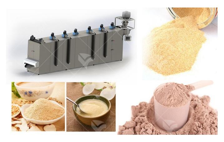
The whole nutrition powder production line can automatically complete the production from mixer, twin screw extruder, air conveyor, multi-layer oven, automatic crash system, blending machine to the finished product.
