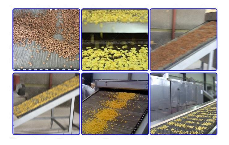
The breakfast cereal production line begins with the breakfast cereal suppliers first putting the raw material into the double screw extruder. The breakfast material, typically a mixture of grains like corn, wheat, and rice, along with other ingredients such as sugar, salt, and vitamins, is then subjected
