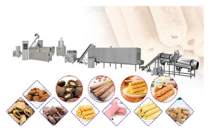
The protein-rich plant material expands into high temperature and short extrusion, the protein is completely denatured, and the tissue structure becomes porous, which is conducive to contact with human digestive enzymes and improves the utilization and digestibility of protein. The puffed snacks product which made by the automatic puffed snacks production line is not easy to regenerate. Due to the regeneration will cause the product to taste rough and the digestibility will be greatly reduced.
