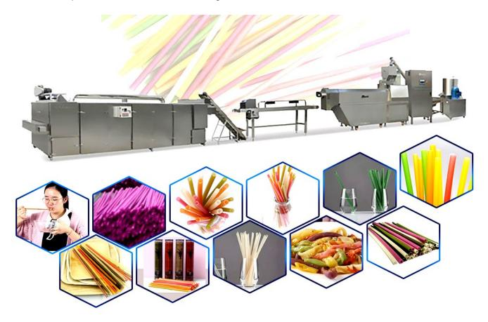
The automatic rice straw equipment is made into blanks of various sizes by a single screw
