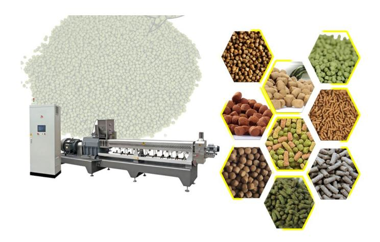
Due to the inherent characteristics of the extruder, the extruded feed product can have a certain degree of puffing effect by adjusting the process parameters of the extruder.
