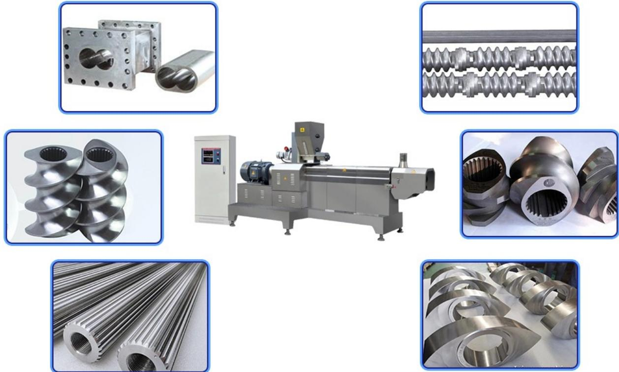
4. When the spiral groove is found to be clogged of the puff making machine, do not stop it immediately. You should run it for a while after stopping the feed, and then stop the machine until there is a burnt smell. This can avoid the sprinkler head and the spiral sleeve from being seized. In case the nozzle and the spiral sleeve cannot be removed due to seizure, don't knock them hard. You can remove them from the body and put them in the fire for a while.
